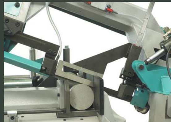
Automatic material sensor minimizes machine setup on semi-automatic models
